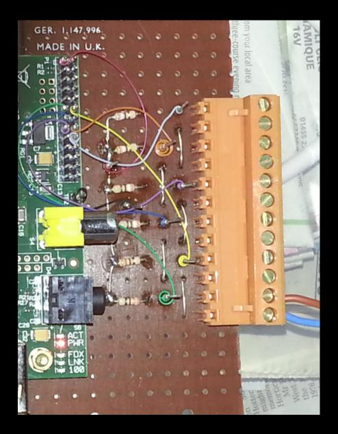
$390\Omega$  pull up resistors (now using  $120\Omega$ ) to the 3.3V rail.
